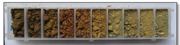
Fig. 6: Chip tray used to store geo-chemical samples.
